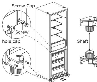
5. Dismantle the screw, sleeve pipe and stopper from the refrigerating door and freezer door, and the support on the lower cover of the refrigerating door is also removed.Then install them on the other side of the doors in order. (Take out the bottom stopperfrom accessories package)
