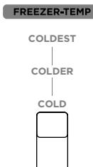
Turn the air damper slider up, the actual temperature inside the freezer room will drop,turn the air damper slider down, the actual temperature inside the freezer room will rise.
