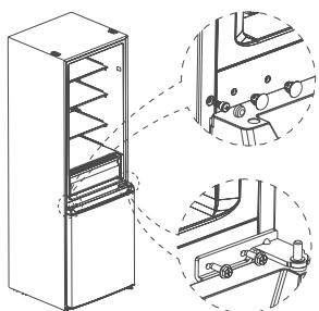
4. Dismantle the bottom hinge, hole caps and screws, on other side of the bottom hinge, then install the hinge on the other side.
