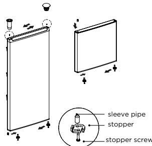
6. Put the freezer door on bottom hinge , install the middle hinge, the screws and the screw hole caps.
